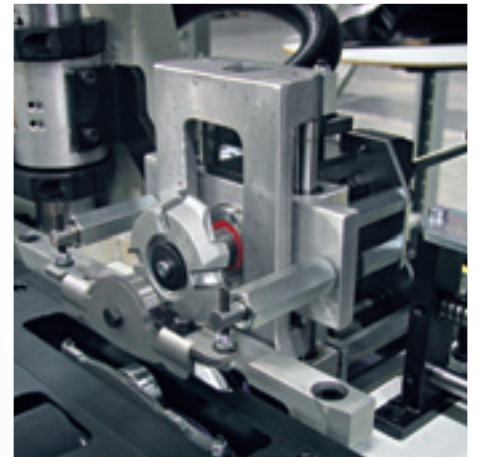
75 mm cutters with shaped profile (2 mm radius)
